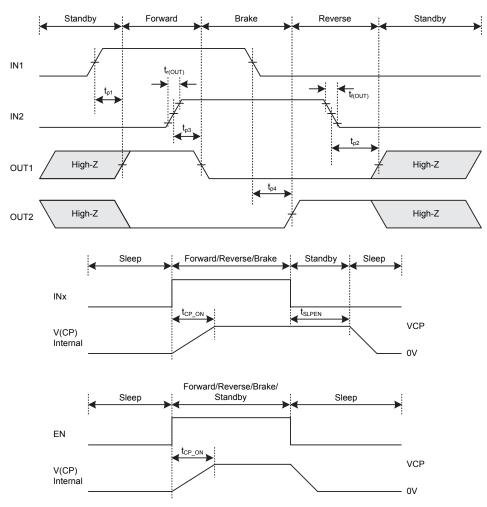
Figure1. Control Logic and Sleep Mode Timing Diagram
